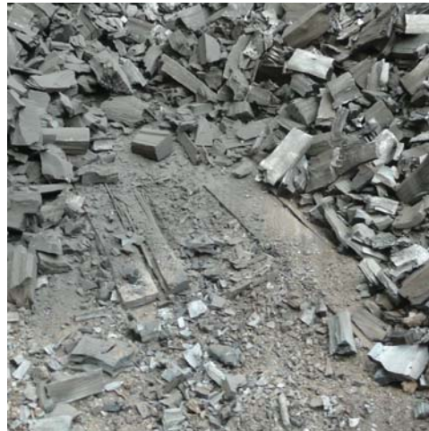
Base construction "Rost" (partly not charred)
