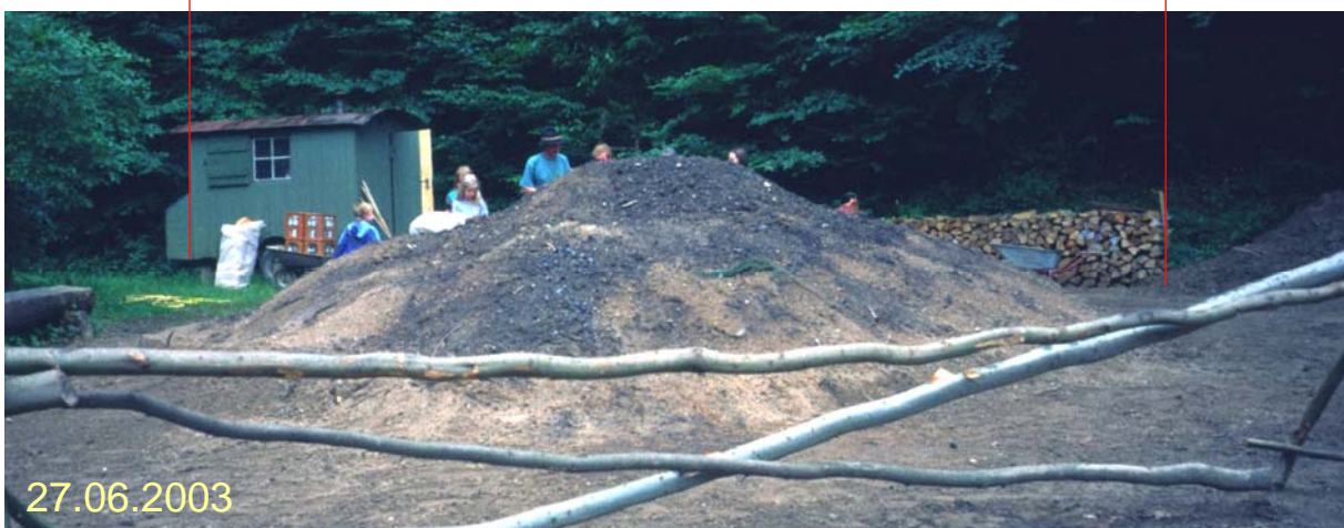
Experimental kiln No.2: Volume reduction (about 50 %) within two weeks (pictures taken exactly from the same field position; cf. red lines)
